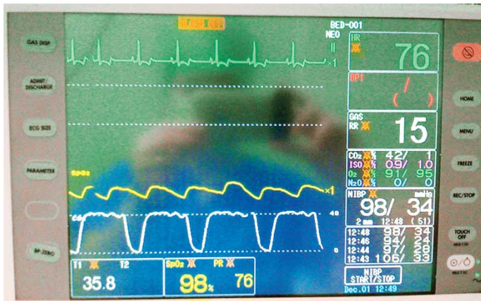
Figure 2. A multiparameter monitor. Note the green ECG trace and heart rate at the top, yellow pulse trace from the pulse oximeter and SpO 2 reading and white capnograph trace with ETCO 2 .
